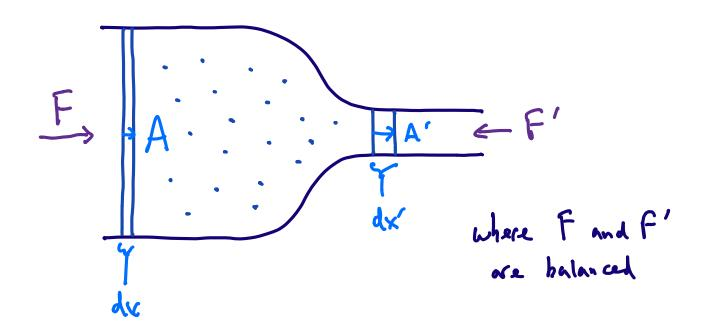
Each piston moves a distance dx and dx, so the corresponding displaced volumes are
